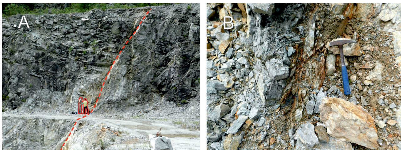
Figure 1.11 A – the N–S oriented fissures and quartz veins (red dashed line) containing carbonate, galena and sphalerite (ankerite) mineralization; B – detail of a quartz vein.
